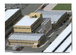
Energy Plastics PVC Compounding plant is located in the modern industrial city of Rabigh, Saudi Arabia. The plant's facilities extend over an area of 4800m<sup>2</sup> and consists of two high-tech PVC compounding lines along fully equipped with sophisticated auxiliary/supporting machinery such as the RM and FG conveying systems, hot and cooling mixers, dosing units, pellet cooling fluidized beds, filling station, ... etc.
